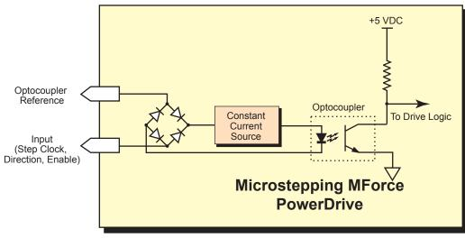
Figure 2.4.4: Optocoupler Input Circuit Diagram
